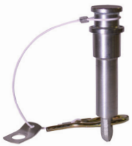
BRADLEY KIT 178 / AL-KO 185013815 25mm Ballpin, Lanyard, Tag, R Clip (less Ball) for V354L 3.5T Universal Coupling
