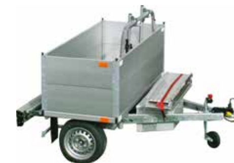
Aluminium side walls 600 mm high on WHEELY
