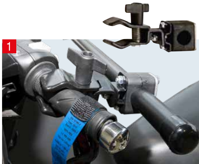
1 Fastening the holding arm with cross clamp on the handlebar
